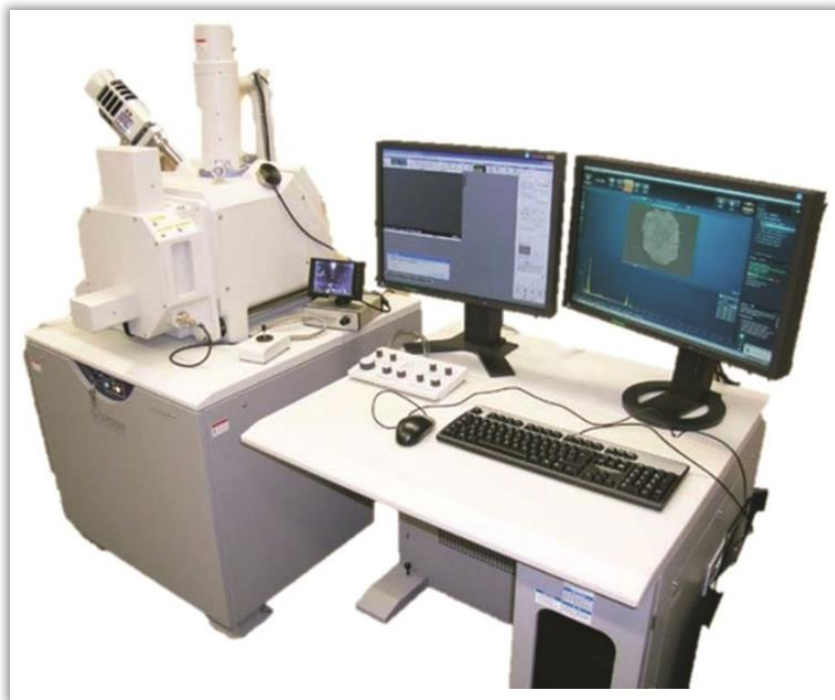
▲ Figure 5. Commercial image of the Hitachi S-3700N scanning electron microscope, pictured here set up to investigate a variety of different tasks.
